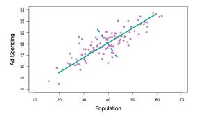
The green solid line indicates the first principal component direction, and the blue dashed line indicates the second principal component direction.
