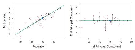
The first principal component direction is shown in green. It is the dimension along which the data vary the most. We get
